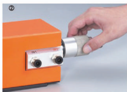
Adjust the size of nozzle according to the diameter of the clamped cable end-sleeves you required.(Increase caliber by twisting clockwise, Decrease caliber by anticlockwise).
